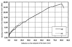
• The load-deflection curves of test beams A1 and A2
