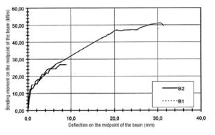
• The load-deflection curves of test beams B1 and B2
