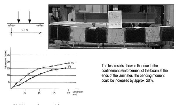
F1: Without confinement reinforcement F3: With confinement reinforcement
