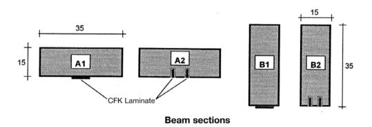
Each sample was either reinforced by a surface-applied CFRP laminate 50/1.2 or by two slot-applied CFRP laminates 25/1.2.
